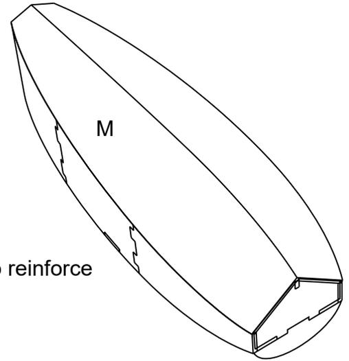
Fill area between ribs with balsa to reinforce
